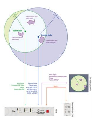
Over wind farms, the RVSE is a unique product that provides ATC with a clear 'radar video' presentation of aircraft tracks, leaving the display free of clutter generated by the turbines http://www.cyrrus.co.uk/wp-content/uploads/2016/09/Cyrrus-RVSE-Tech-Sheet.pdf. In areas where PSR coverage is poor, the RVSE is a cost-effective method of integrating the radar picture with an alternative radar source.
